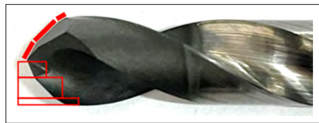
Figure 2. SDC drill bit.
