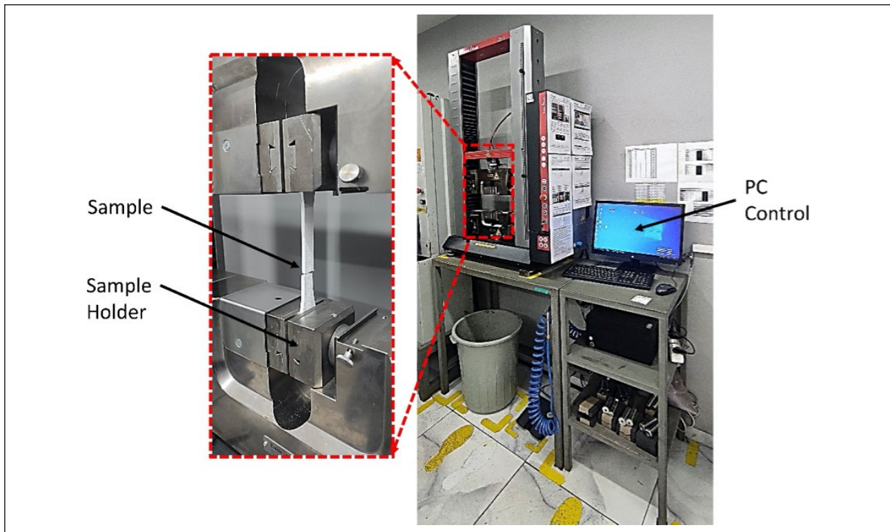
Figure 4. Tensile test experimental setup.
