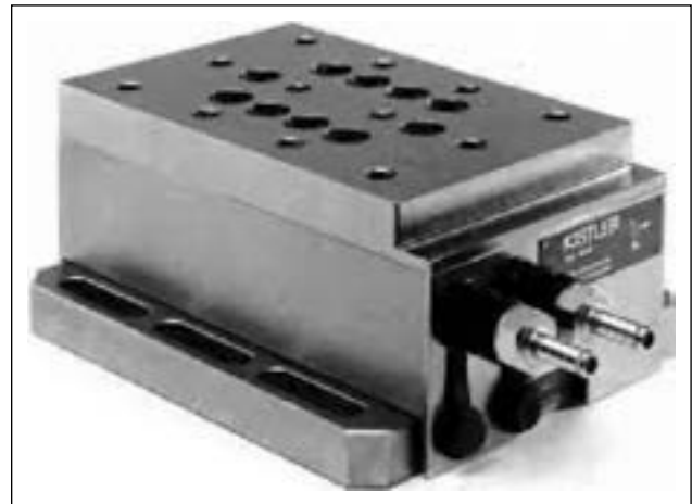
Figure 4. Kistler 9257B dynamometer [24].
