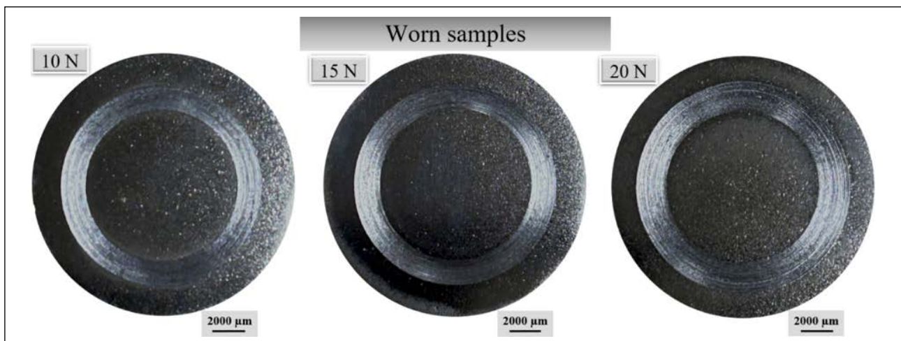
Figure 2. Macro images of the worn samples.
