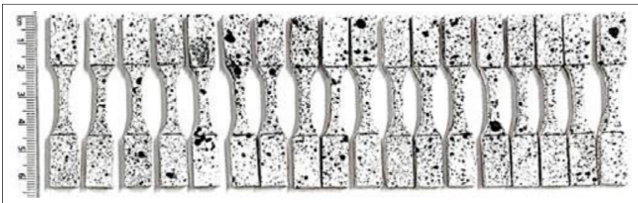
Figure 2. Surface spackle pattern preparation of tested 18 specimens.
