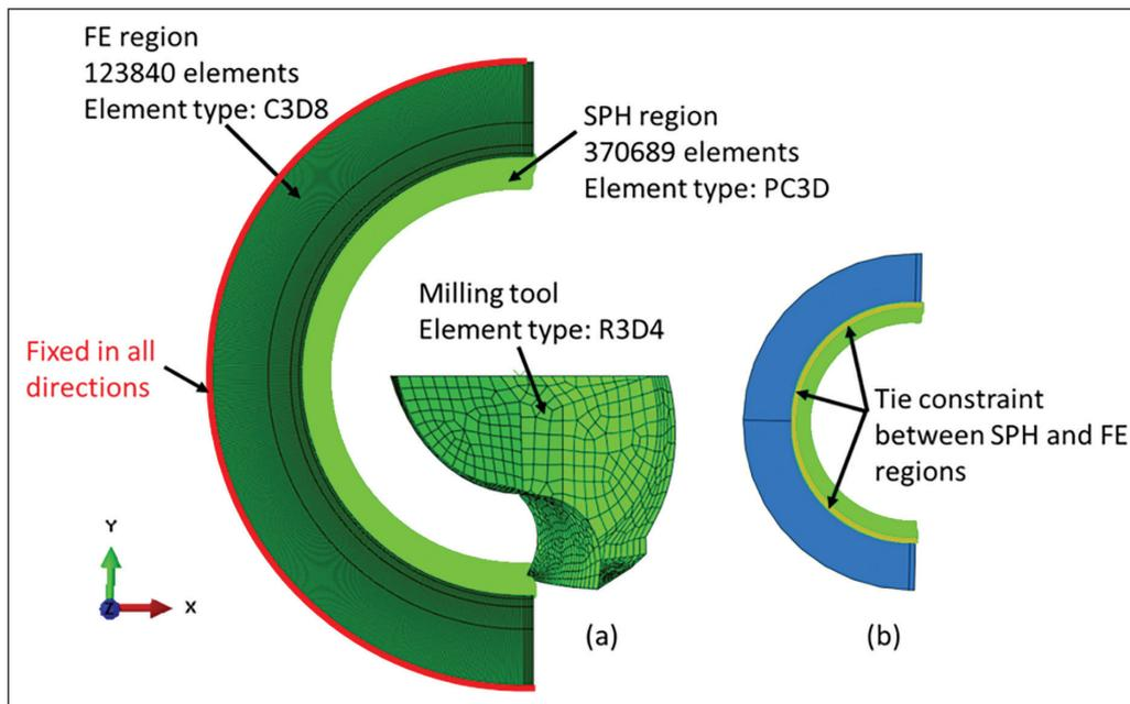
**Figure 1.** (a) 3D SPH-FE model of micro-milling of Ti alloy (b) Details of tie constraint imposed.
