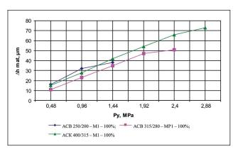
**Figure 3**. Dependence of linear removal on pressure during sliding of a 50 steel specimen with a hardness of HB=188 on an abrasive surface.
