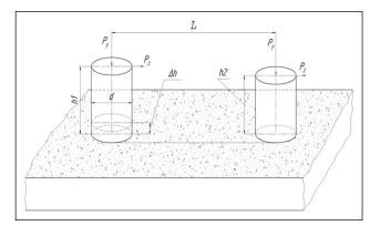
**Figure 1**. Scheme for determining the cutting ability of a diamond bar at processing of various materials:  $P_y$  – radial cutting force, MPa;  $P_z$  – tangential cutting force, MPa; d – diameter of the test material sample, mm;  $h_1$  and  $h_2$  – sample height, respectively, before and after processing, mm;  $\Delta h$  – the amount of linear material removal, mm; L – length of the path traversed by the sample on the abrasive surface, mm.
