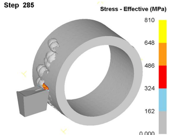
Figure 9. Effective stress of elliptical chip breaker.
