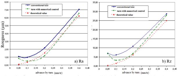
**Figure 3.** Influence advance by turn on roughness (Vc = 180 m/min, ap = 1 mm, R $\epsilon$  = 0.8 mm) a) Ra, b)Rz
