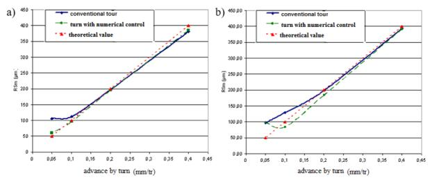
**Figure 5.** Influence advance by turn on RSm roughness a)  $r_{\varepsilon} = 0,4$  mm, b)  $r_{\varepsilon} = 1,2$  mm (Vc = 180 m/min, ap = 1 mm, Rå = 0,8 mm)
