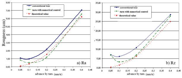
**Figure 2.** Influence advance by turn on roughness (Vc = 180 m/min, ap = 1 mm, R $\epsilon$  = 0.4 mm) a) Ra, b)Rz
