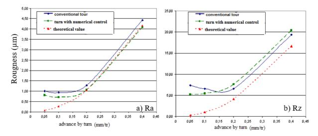
Figure 4. Influence advance by turn on roughness a) Ra, b) Rz (Vc = 180 m/min, ap = 1 mm,  $R\epsilon = 1.2$  mm)
