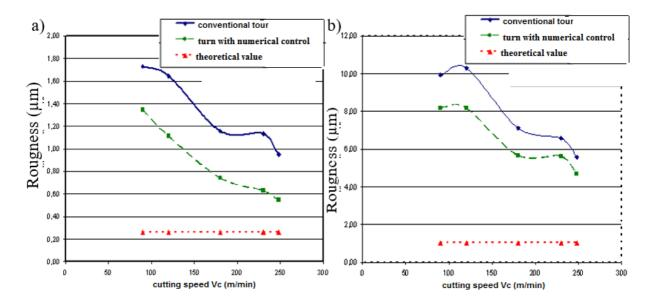
Figure 6. Influence cutting speed on roughness a) Ra, b) Rz (f=0.1 mm/tr, ap = 2 mm, rå = 1,2mm)
