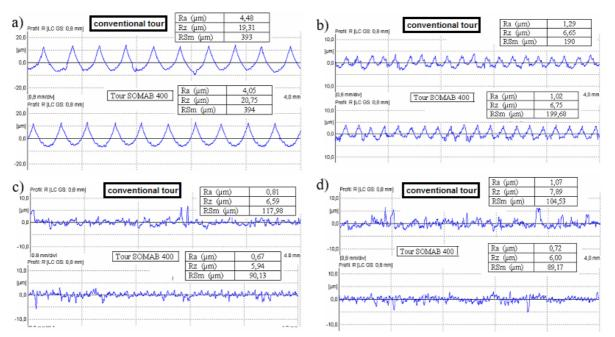
**Figure 1.** Status returns of surface, for the advances by tour (Vc=180 m/min, ap=1 mm,  $R_{\epsilon} = 1.2$ mm) a) f= 0,4 mm/tr, b) f=0,2 mm/tr, c) f=0,1 mm/tr, d) f=0,05 mm/tr
