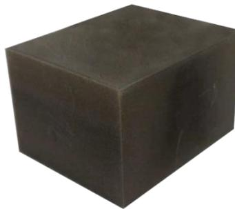
**Figure 1.** The image of specimen produced by DMLS method
